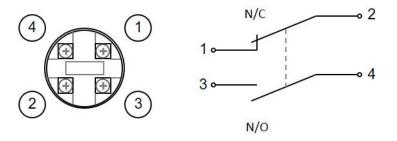
The switch is not polarity sensitive
