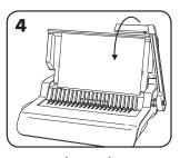
4. Test punch scrap sheets to check edge guide setting.
