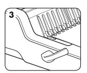
3. Load punched sheets directly onto the opened comb. Starting with the front of the document.
