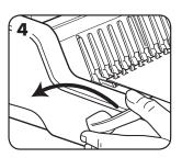
4. When all punched sheets are loaded onto the comb, push the comb lever backwards to close the comb and remove the bound document.
