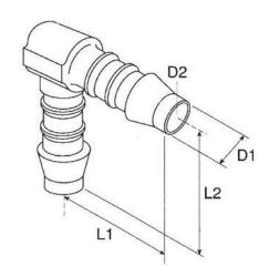
D1: Joiner Outer Diameter D2: Joiner Inner Diameter
