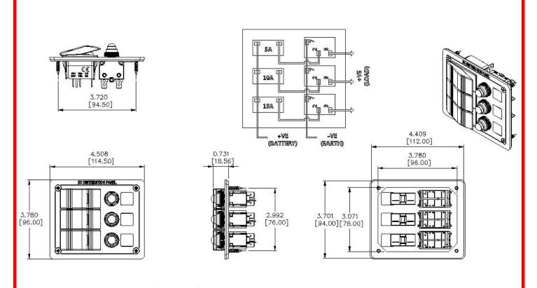
Rocker Switch x 3 (SPST / ON-OFF) 5A Breakers x 1 10A Breakers x 1 15A Breakers x 1 Rubber Pad x 1 Stainless Steel Screw x 4 Symbol x 40 option Size of Panel: 114.5x96mm Size of Screw Hole: 94.5x76mm Size of Hole: 86x72mm
