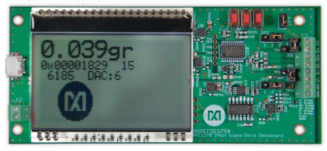
3. Upon power-up, the board will take 10 measurements and display the ADC LSB value during this process. These 10 measurements will be averaged and the average will be used as the zero-position.
