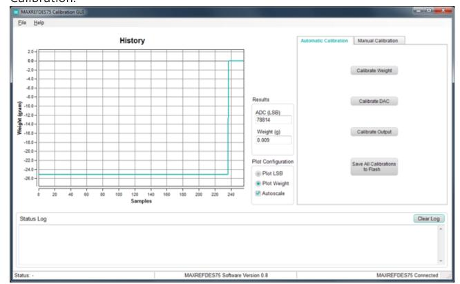
The recommended process is to use the "Automatic Calibration" tab, which leads the user through the entire process. The calibration factors established by the automatic calibration are populated in the appropriate text boxes in the "Manual Calibration" tab and can be reviewed after calibration.
