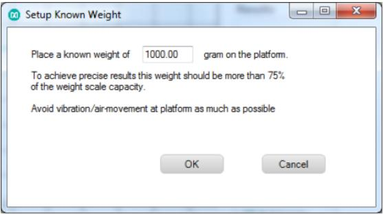
12. The MAXREFDES75# will take 10 measurements while the known weight is placed on the platform and shows the progress.
