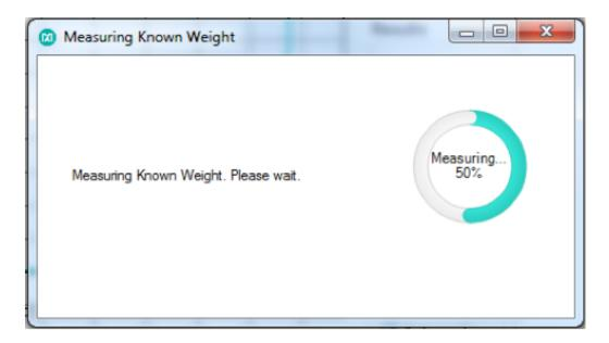
13. After the second measurement, the MAXREFDES75# calibration GUI will calculate the offset and weight factor and send the results to the MAXREFDES75# board. The results are also populated in the appropriate text boxes in the "Manual Calibration" tab.
