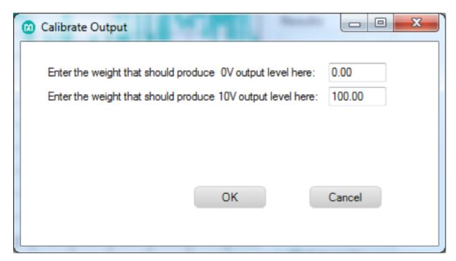
19. Verify that the weight scale now measures weight accurately and that the analog output changes appropriately.
