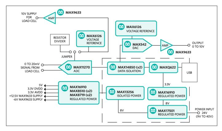
The signal chain begins with the sensor signal feeding directly into the MAX11270. No external op amp is necessary because the PGA is integrated in the MAX11270. Following isolation via the MAX14850, the MAXQ622 reads the input signal, applies zero-offset and weight-factor, and presents the resulting weight. The MAXQ622 calculates a DAC value, based on DAC calibration and output range mapping and writes this to the DAC. A variety of sensor power options are available, outlined in **Table 1**.
