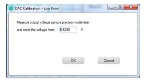
16. The MAXREFDES75# will generate DC 9.375V. Measure the exact result with the multimeter and enter the measured result into the text box and click the "OK" button.
