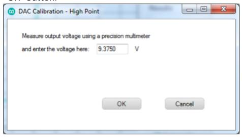
17. After the second measurement, the MAXREFDES75# calibration GUI will calculate offset and gain for the analog output and will send the results to the MAXREFDES75# board. The results are also populated in the appropriate text boxes in the "Manual Calibration" tab.
