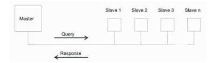
In the Modbus™ Protocol the master can address individual slaves, or, using a special "Broadcast" address, can initiate a broadcast message to all slaves. The 236-9299 digital power measurement meter does not support the broadcast address.
