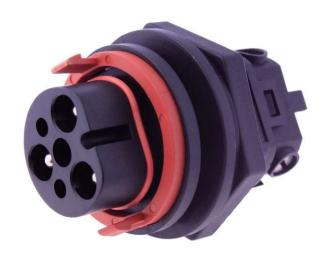
The RS PRO series of waterproof power connectors are ruggedly built connectors sealed to an IP67 rating with a push-lock coupling which requires the series coupling tool to remove. This provides a more secure connection ideal for use when electrical safety or tampering may be an issue. The M35 range of connectors are designed with 3 gold plated contacts rated to 41A at 600V and are available in panel to cable or cable to cable variations.
