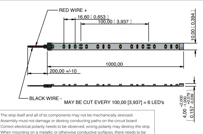
electrical isolation points between strip and the mounting surface.
