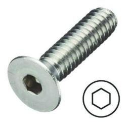
Countersunk socket screws are designed for light duty applications where there is limited space. These screws are widely used in many applications where a strong and reliable joint is required. Typically countersunk socket screws are used to fasten plates and strips of metal to equipment and machinery as their flat head allows a flush flat finish. This range of socket screws is bright zinc plated and is suitable for indoor and dry environments.
