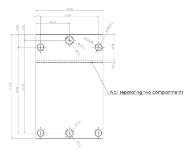
Dashed line shows outline of the mounting boss under PCB board Recommended mounting holes diameter Ø3,5mm All dimensions are given within +/-0,5mm tolerance
