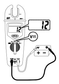
▲ Warning Do not apply more than 600V rms dc between the instrument terminals and earth ground .
