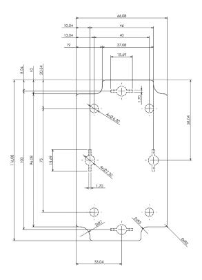
Dashed line shows outline of the mounting boss under PCB board Recommended mounting holes diameter ø4mm All dimensions are given within +/-0,5mm tolerance
