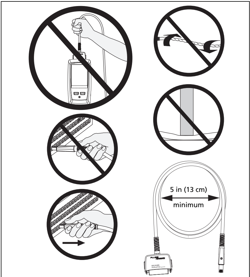
Figure 24. How to Prevent Damage to the Permanent Link Adapter Cables
