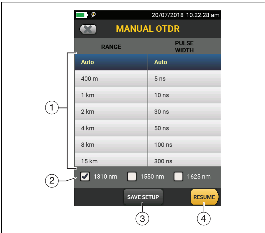
Figure 161. Manual OTDR Screen for Quick Changes to Settings in Real Time Trace Mode
