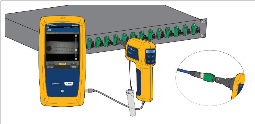
Figure 107. Inspect an Endface (FI-3000 shown)
