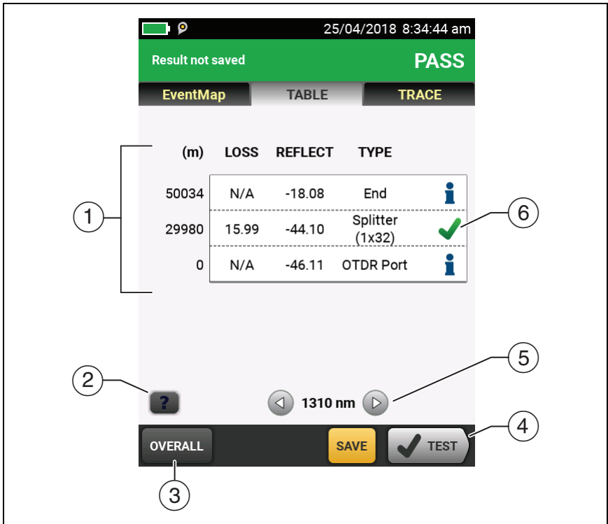
Figure 180. Event Table from an HDR OTDR Test
