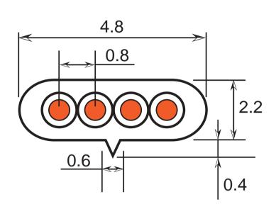
Flat black telephone cable, composed of 4 conductors 28 AWG.
