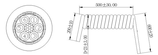
Cable Making: RS PRO 6x0.14mm<sup>2</sup> Coiled Data Cable
