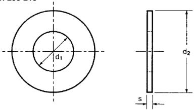
This RS Pro range of hard rolled copper washers are generally used with a machine threaded fastener and nut to spread the load over a greater surface area when tightening a bolt, screw or nut.
