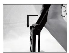
3. Lock core in place by pushing against the latch at one of three height calibrations.
