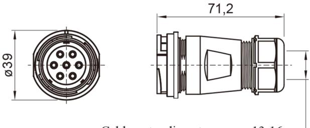
Cable outer diameter range: 13-16mm
