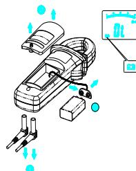
**⚠ Warning :** Disconnect the clamp-multimeter from all power sources and remove it from around a conductor before removing the battery compartment cover.
