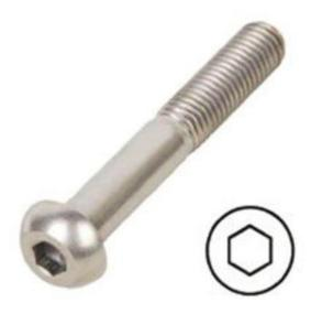
Button Head Socket Screws are designed for light duty with a similar thread design as a Socket Cap Screw although the dome shaped head is wider and has a lower profile than a Socket Cap Screw, presenting an aesthetic appearance to an assembly.
