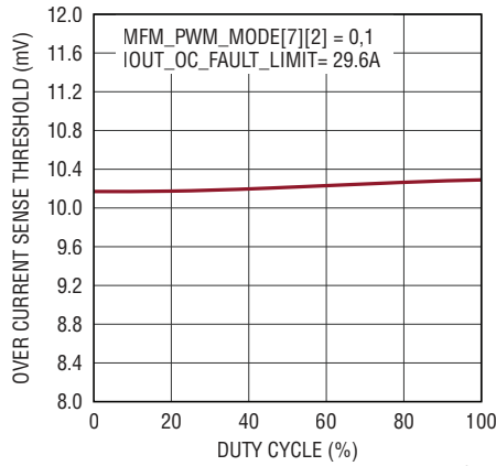
Current Sense Threshold vs Duty Cycle
