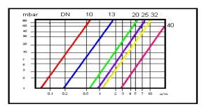
Schedule 2: Pressure loss for type of end connection based in internal diameter (DN)
