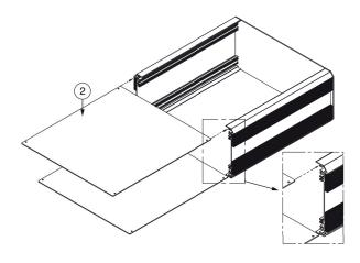
3. Slide the ② top/bottom covers into the side frame slots.
