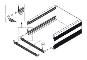
2. Install (6) GP Bar Kit [option] into the slide rail slot in side frame and secure with GP Bar position by Umbrella Phillips Screw M5-10 (Dog Point). We advise to install user components at this stage. Our GP Bar Kits are ideal for this purpose, but user can prepare their own method.
