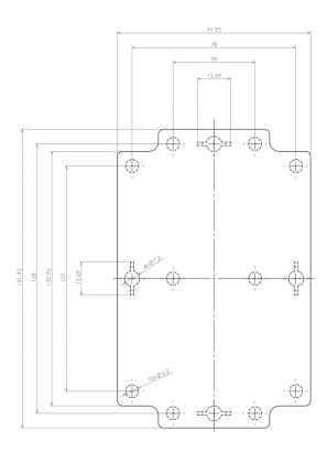
Dashed line shows outline of the mounting boss under PCB board Recommended mounting holes diameter Ø4mm
