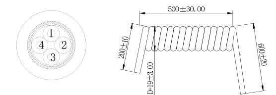
Cable Making: RS PRO 4x0.14mm<sup>2</sup> Coiled Data Cable
