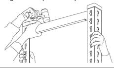
To locate beams: Clip lugs at the ends of the beam into the 'P' slots in the upright. Press down, then tap into place ensuring lugs are fully located to the base of the slots.
