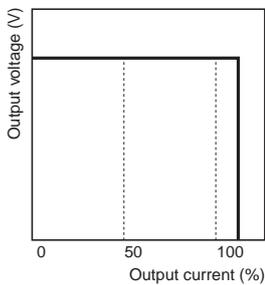
\*1. Operation is intermittent in a fixed cycle in short-circuited or overcurrent states.
