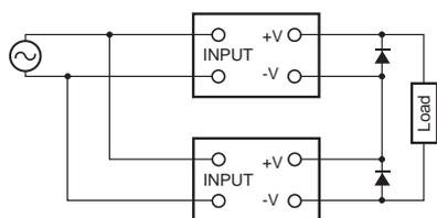
**Note: 1.** The diode is connected as shown in the figure. If the load is short-circuited, a reverse voltage will be generated inside the Power Supply. If this occurs the Power Supply may possibly deteriorate or be damaged. Always connect a diode as shown in the figure. Select a diode having the following ratings.
