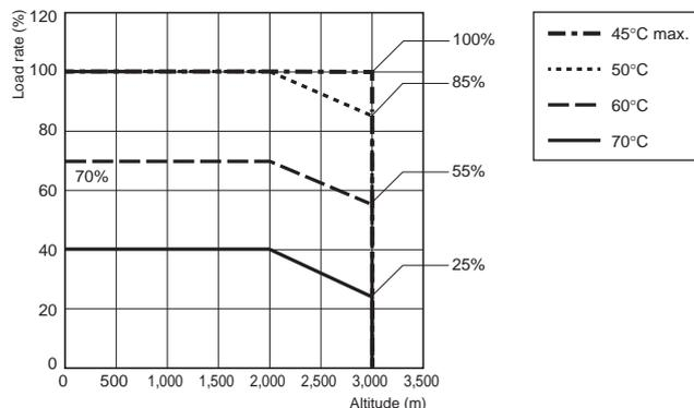
**Note:** At a voltage below 100 VAC, reduce the load at the rate of 1.3%/V. (40°C < Ambient temperature ≤ 70°C)
