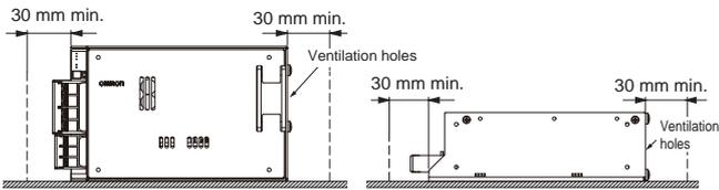
**Note:** Use a metal plate as the mounting surface.
