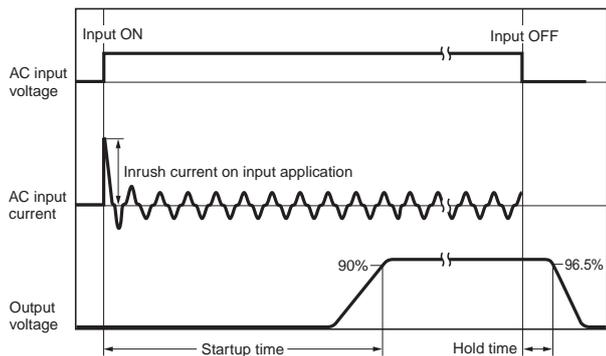
**Note:** The total inrush current of all of the Power Supplies will flow for parallel operation or backup operation. Sufficiently check the fusing characteristics of fuses and the operating characteristics of breakers and select fuses and breakers so that external fuses will not burn out or breakers will not operate due to inrush current.
