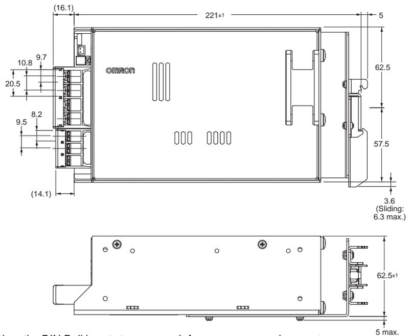
**Note:** Use a Front-mounting Bracket (S82Y-FSG-60F) when the DIN Rail is not strong enough for your usage environment.
