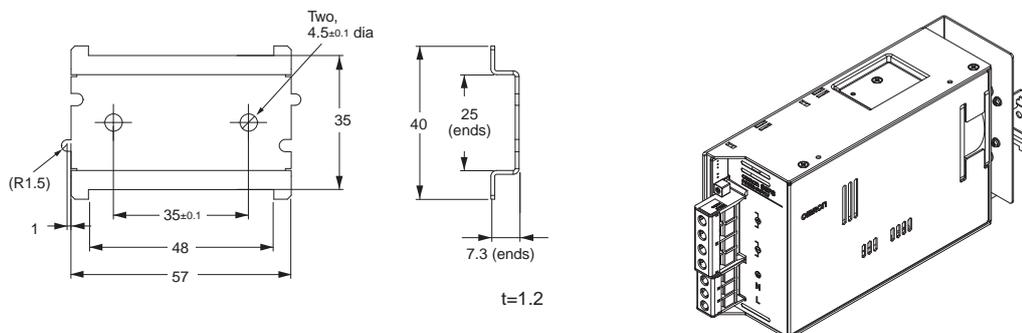
**Note:** Replacement brackets from the S8JX-N, S8JX-P, and S8VM series are available. Use these brackets for a front mounting configuration using direct mounting models. Refer to the data sheet (Cat. No.: T216-E1, T217-E1, and T218-E1) for more information.
