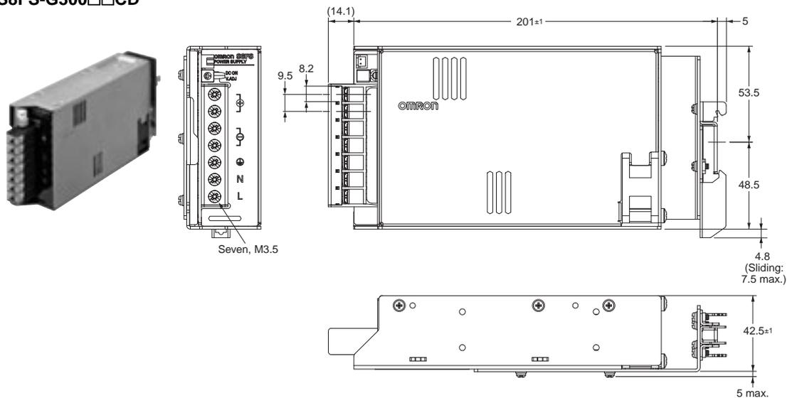
**Note:** Use a Front-mounting Bracket (S82Y-FSG-30F) when the DIN Rail is not strong enough for your usage environment.
