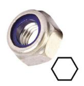
Nylon Insert Lock Nuts are Hex Nuts that have a captive nylon washer mounted in their top to create a prevailing torque type Lock Nut. The undersized washer forms a compression grip that binds on the threads of the mating fastener to resist loosening.
