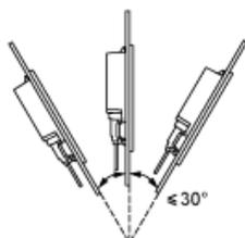
When installing the panel in a slanted position, and the panel face inclines more than 30°, the ambient temperature must not exceed 40 °C (104 °F).
