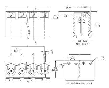
Positions: 02 thru 24 A = .197 [5.00]x No. of Positions B = .197 [5.00] x No. of Spaces
