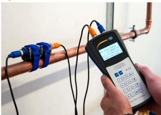
The PCE-TDS 100H ultrasonic flow meter measuring a pipe.
