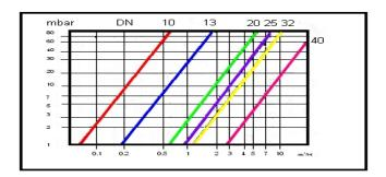
Schedule 2: Pressure loss for type of end connection based in internal diameter (DN)
