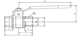
DN shows the nominal flow diameter. Actual flow diameter complies with full port DIN 3357 part 4. Stem configuration of valves over 2" is slightly different.
