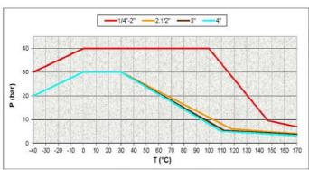
AS4617 Limitations for GAS: 2100 Kpa up to 2" and 1500 Kpa from 2. 1/2" to 4" rated working pressure and 0°C +60°C temperature
