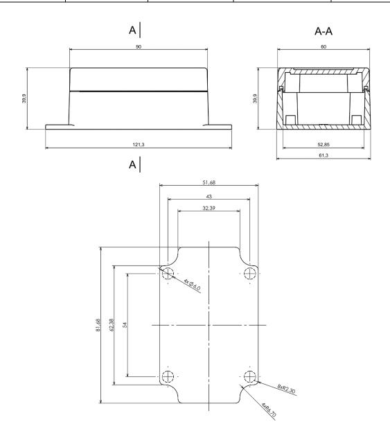
Dashed line shows outline of the mounting boss under PCB board Recommended mounting holes diameter Ø4mm
