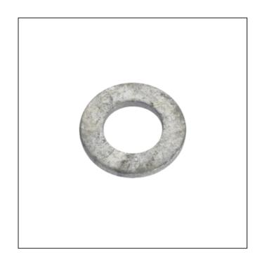
Used with threaded fasteners (for example a bolt and a nut), designed to increase the area of load distribution. When the threaded fastener is tightened, there is a risk of the surface (or surfaces) becoming stressed. A washer helps spread the tightening forces applied over an even and increased area, reducing the risk of surface stress and damage. These washers conform to DIN 125A and are made of steel. The galvanised finish offers great resistance to corrosion.
