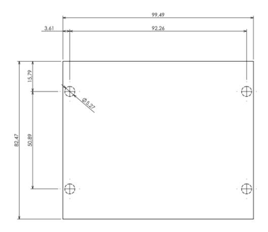
Dashed line shows outline of the mounting boss under PCB board Recommended mounting holes diameter Ø3.5 mm All dimensions are given within +/-0,5mm tolerance
