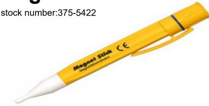
The Magnet Stick is an instrument for testing the presence of magnetic fields. By simply holding the tip of the instrument near the test area, it indicates a magnetic field by glowing. The test lamp responds to all kinds of magnetic fields, from alternating current to direct current and permanent magnets. (Sensitivity 30 gauss 3 mT)
