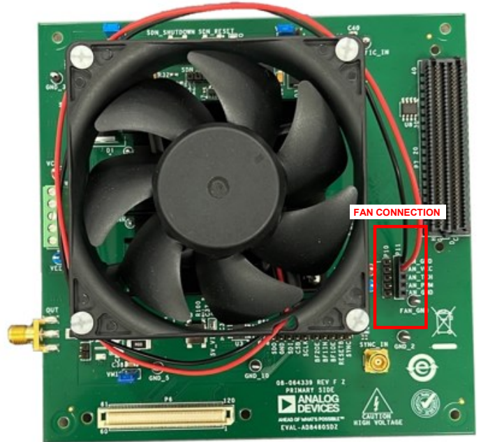
Figure 9. AD8460 Evaluation Board with Fan Attached
