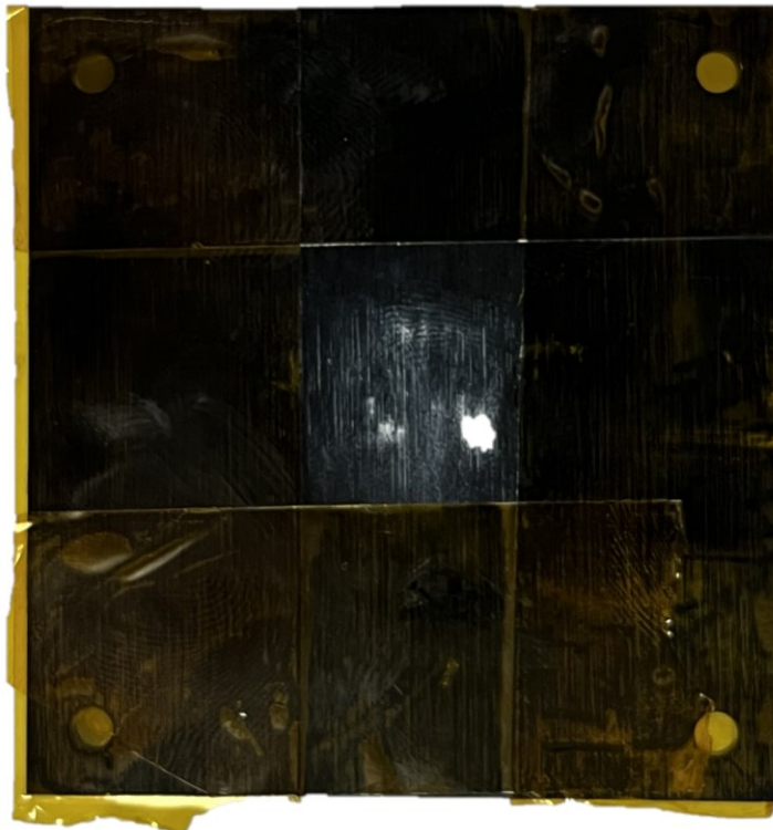
Figure 6. Back of Heatsink with Kapton Tape
