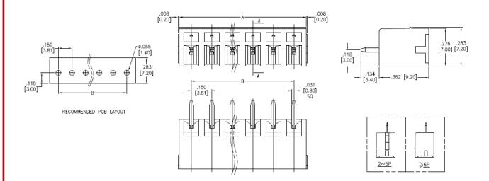
Positions: 02 thru 24 A= .150 [3.81]  $\times$  No. of Spaces + .181 [4.60] B= .150 [3.81]  $\times$  No. of Spaces
