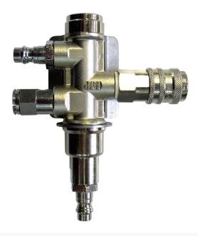
**SWOV** is an automatic switching device of the air feeding source, from air network to back-up breathing apparatus (**SEKUR NAVY MASK**) which intervenes in case the air line should stop or its pressure significantly drop.
