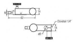
Indicator fitting is 8 mm in diameter including the dovetail
