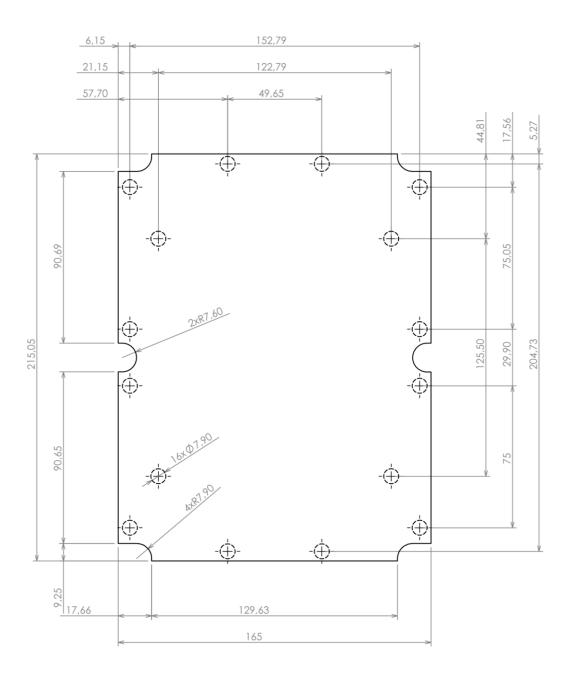
Dashed line shows outline of the mounting boss under PCB board Recommended mounting holes diameter ø3,5mm
