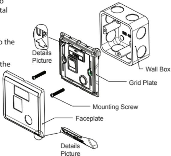
Insert a screwdriver into the clip lock, and twist the screwdriver to remove the faceplate.
