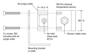
Two M3 screws (included) secure both the air purge collar and the sensor to the mounting.
