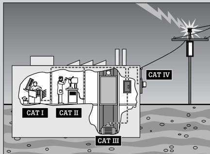
To protect your instrument and –more importantly– yourself, choose a test tool that can withstand the electrical hazards present in the environment in which you plan to use it. EN61010 establishes international safety requirements for electrical measurement equipment. It separates the various electrical environments into installation categories based on the danger from high voltage-energy
