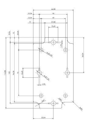
Dashed line shows outline of the mounting boss under PCB board Recommended mounting holes diameter Ø4mm All dimensions are given within +/-0,5mm tolerance
