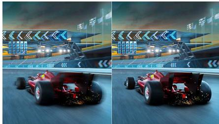
In an effort to reduce motion blur, this monitor's LED backlight will work simultaneously with the refresh rate to control brightness levels for the best picture clarity. Please note that Smart MBR is a type of gaming mode and it is recommended to turn the function off when not gaming as it may cause screen-flickering.
