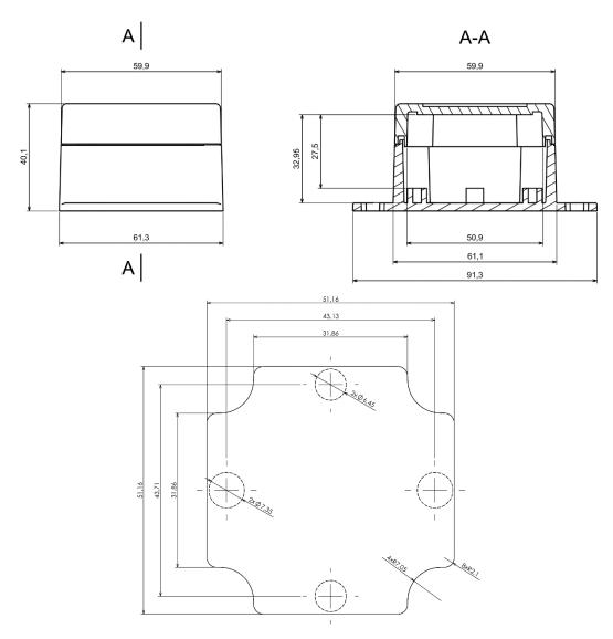
Dashed line shows outline of the mounting boss under PCB board Recommended mounting holes diameter ø4mm All dimensions are given within +/-0,5mm tolerance
