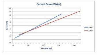
Pressure shown is the not to exceed value. All MG2000 pump variants are capable of more than the indicated figure but exceeding this may result in damage to the pump.
