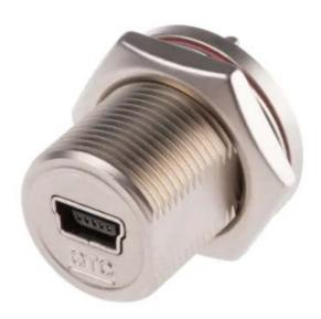
The RS PRO series of waterproof Mini USB-B connectors are a range of ruggedised IP67/IP68 connectors designed to be used outdoors or in harsher industrial environments. Designed to fit panel cut outs of 16mm the metal Mini USB-B series also comes with rear potting on the panel mount connectors. This ensures your panel is still sealed to an IP67/IP68 rating even when the connector is unmated, and the sealing cap is not connected. The bayonet or screw mating allows for a secure connection.
